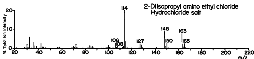
Fig. 6. Pyrolysis mass spectrum of 2-diisopropylaminoethyl chloride hydrochloride. Note the presence of peaks which are also present in the spectrum of the insoluble fraction of Biomer [Fig. 3(B), m/z 106/108, 114, 127, 148/150, and 163/165].
